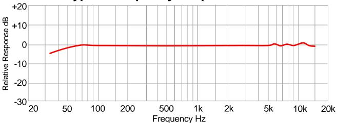
**Sensitivity:** -66dB ±3dB (0dB=1V/uBAR@1kHz)
